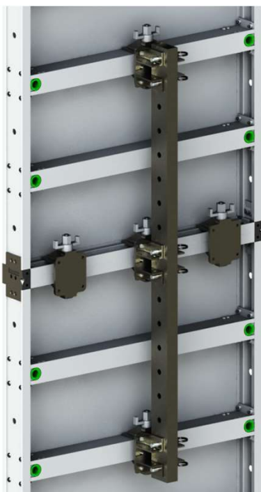
Figure 4. Place Alignment Bar Stacking Assembly At Or Near The Center Of The Panel Width & Attach Standard Clamps On Either Side
