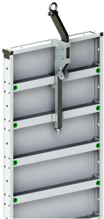
Figure 5. Place Stacking Clamp / Lifting Bar In Any Position Between The Siderails And No Closer Than 6" To The Edge Of The Panel
