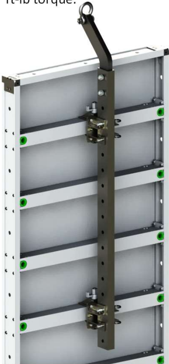
Figure 4. Place Alignment / Lifting Bar In Any Position Between The Siderails And No Closer Than 6" To The Edge Of The Panel
